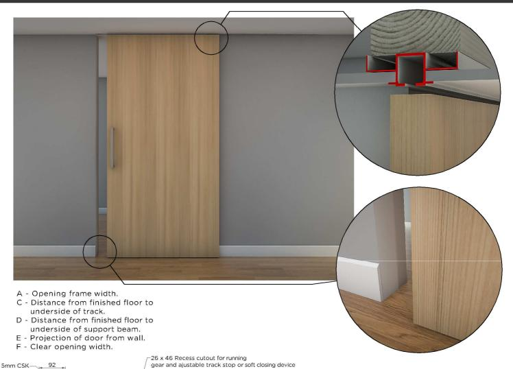
Suspension mounting plate must be RECESSED into the door
